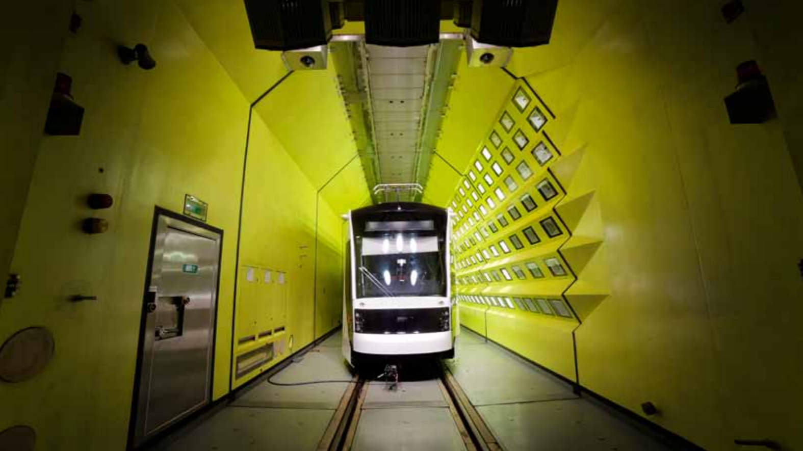
Siemens Avenio People Mover System for Qatar Foundation's Education City undergoing climate chamber testing in Wegberg Wildenrath, Germany
