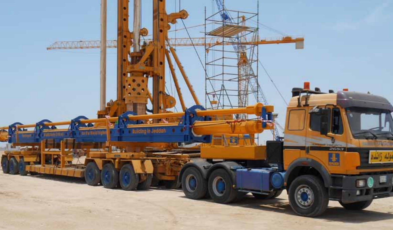
The longest Bauer Kelly (110 m) for the world's highest building in Jeddah
